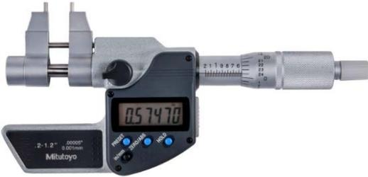
**345-350-30 DIGIMATIC CALIPER JAW TYPE ID MICROMETER**, carbide steel tip, locking clamp, ratchet stop, with SPC data output
