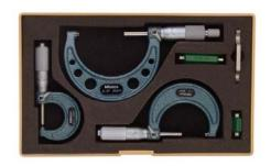
**103-922 OD MICROMETERS,** 3pc set with standards. 0-" and 1-2" have friction thimble, 2-3" has ratchet thimble
