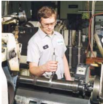
Virtually any kind of machined feature can be measured for dimension, position, clearance and interference, and form errors.
