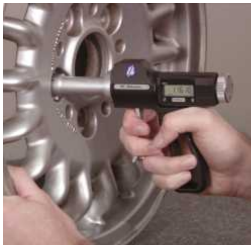
Pistol-grip bore gages are very adaptable to measuring special features such as spline pitch diameter, ball races, and ball nuts.
