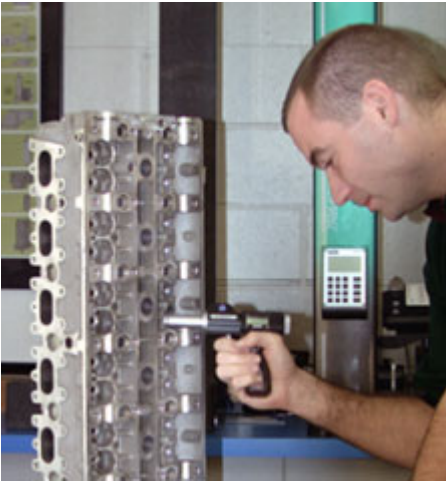
spherical anvils help adjust for axial gage head misalignments of up to \pm 10 degrees
